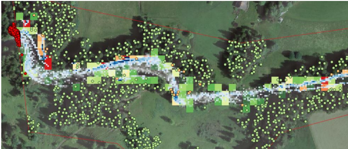
Figure 10: Example of the spatial results. The point shapefile "trees_end.shp" represents all trees at the end of the simulation. Green= rooted living wood, orange= deposited wood, red= wood at LSB. The coarse raster "Mobilisation_volume.tif" shows the volume of the mobilized wood in each raster cell. The fine raster "Flowpath_volume.tif" shows the volume of woody material which flew over each raster cell. Orthoimage: swisstopo
